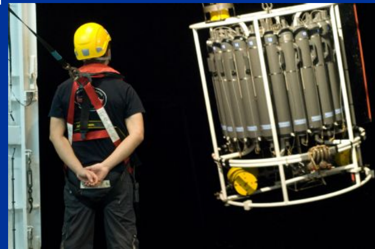
CTD 911 + and rosette with LADCP installed
